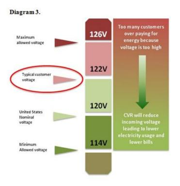
Lacking real-time operating information at the meter, utilities generally deliver energy at a conservative 120V to account for distribution line losses that could cause the voltage delivered
